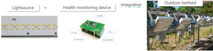
Fig. 13.25 System integration into an outdoor test bed
