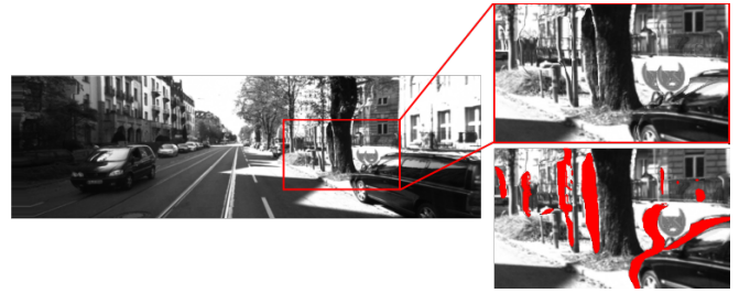
Fig. 4. Double-mapping artifact from image reconstruction, and the masked out areas after validity check
