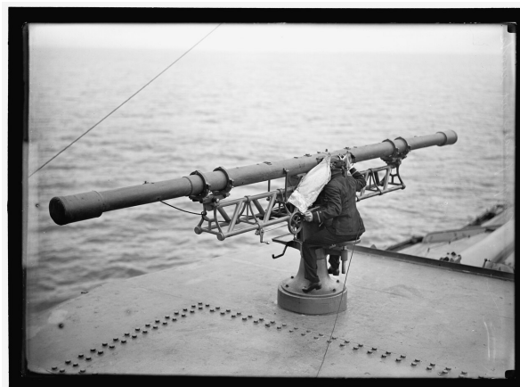
Figure 3.1: The principles of disparity in stereo vision has been harnessed for depth estimation for much longer than the emergence of computer vision. "Target practice. Range finder at work." by Harris & Ewing, 1913 2
