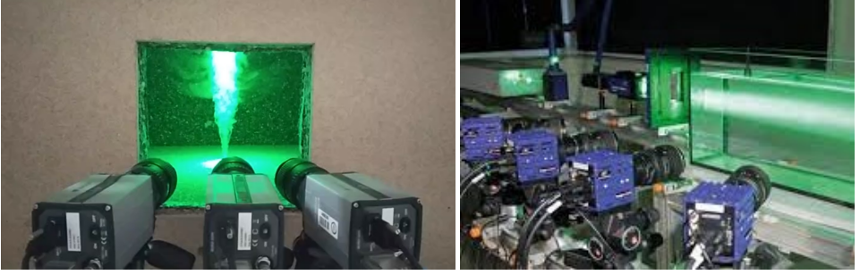
Figure 2.8: Typical TOMO PIV setups with several cameras. Left: 3-camera setup for jetflow measurements, from Nextflow project: https://erc-nextflow.uc3m.es/the-project/ . Right: 4-camera system for water flows measurements, from LaVision : https://www.lavision.de/en/products/flowmaster/tomographic-piv/ .
