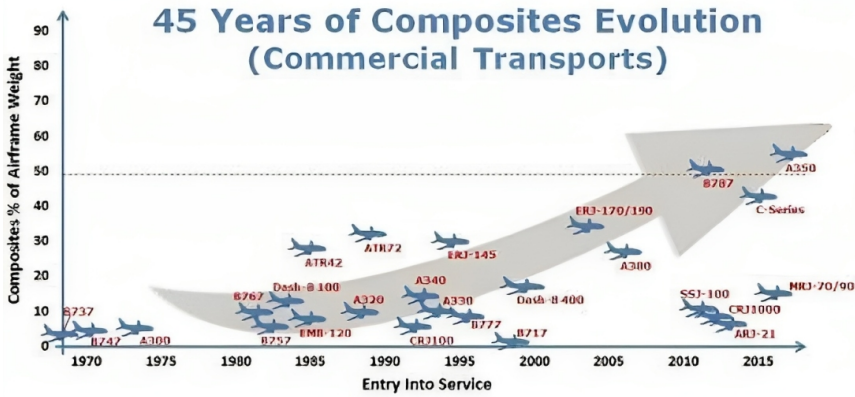
Figure 1.3: Evolution of composite materials in aviation. Figure adapted from Composite World : http://www.compositesworld.com/blog/2014 .
