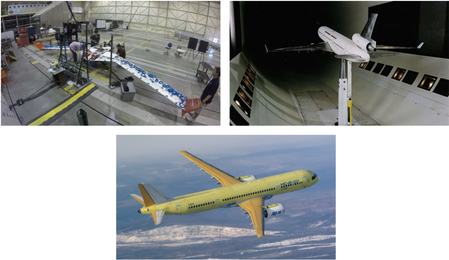
Figure 1.7: Wind tunnel tests (top-right), ground vibration test (top-left) and flight flutter test (bottom).
