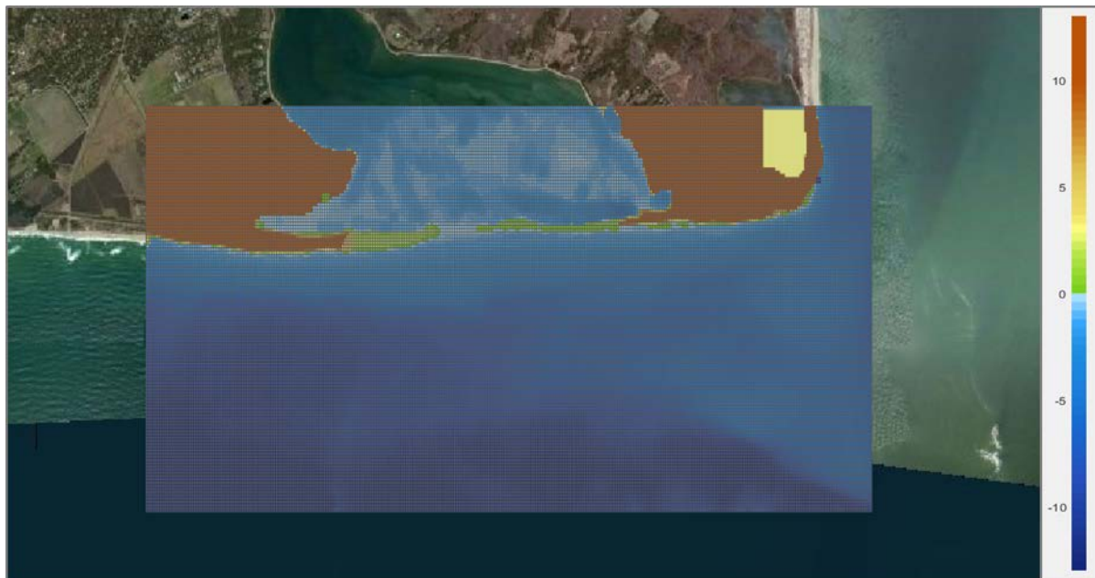
Figure E.4. Initial near-equilibrium bathymetry used in all the simulations in Katama Bay.
