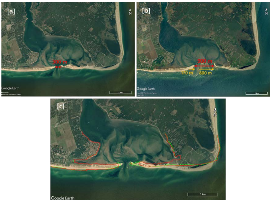
Figure 3.14. Satellite images of the validation period; July 2007 (a) and July 2008 (b). Red arrows illustrate the inlet width, whereas orange arrows indicate the inlet barriers migration. Initial inlet bathymetry (green contour line) and after the validation simulation (red line). Satellite images from (Google Earth 2018a).
