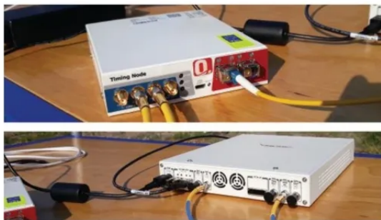
FIGURE 3 WR timing node (top) fed by a 1.25 gigabit per second bitstream through an optical fiber (yellow cable to the right) and providing electrical 1 pulse per second and 10 MHz synchronization signals at the outputs (two cables to the left). The bottom image shows an SDR system. The two channels of this device, capable of wideband operation, act here as a wireless transmitter or as a receiver. The transmitters are synchronized to the WR network through the 1 pulse per second and the 10 MHz electrical signals (blue-yellow cables at bottom) provided by the WR timing node.
