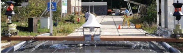
FIGURE 5 Receiver antenna mounted on the roof of a car. Two 360° prisms are used to determine the receiver ground-truth positions at the millimeter level, by means of land surveying total stations (placed on the yellow tripods in the distance).
