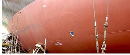
Figure 1.4: ICCP anode and shield around it, obtained from [6].
