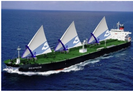
Figure 2.2: Delta wing sails of Seagate Sail (IWSA, 2016)
