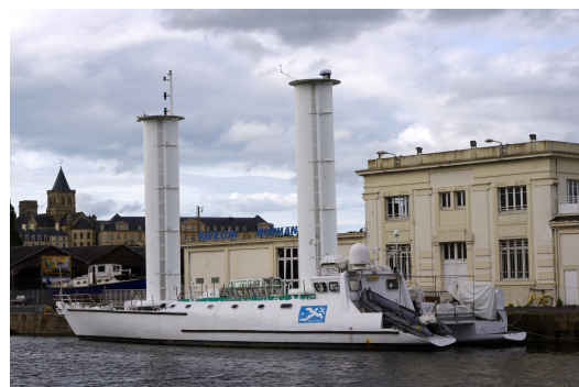
Figure 2.9: Alycone - the Jacques Cousteau's Turbosail ship (Cousteau, 2011)
