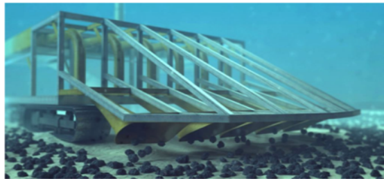
Figure 1.1: Allseas plans to scoop polymetallic nodules from the sea floor (Mining Magazine, 2019)
