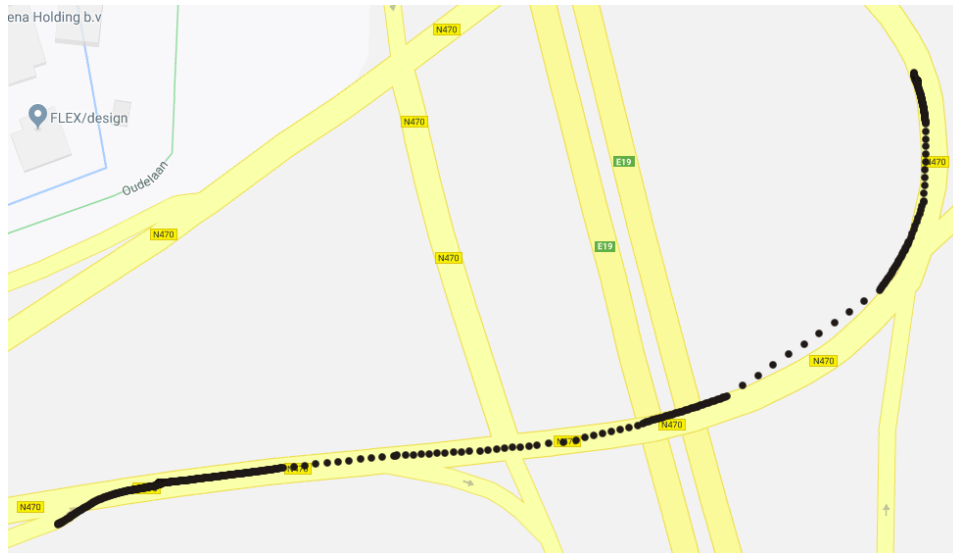
Fig. 6.1: Location data gathered while driving around Delft, laid over Google Maps. The spots with less frequent dots is where the GNSS sensor fails.
