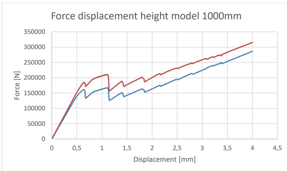
Figure 80 Force displacement diagram of the 2D model with a height of 1000mm and two layers of reinforcement
