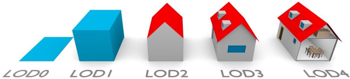
Figure 1: LOD specification [Biljecki et al. (2016)]
