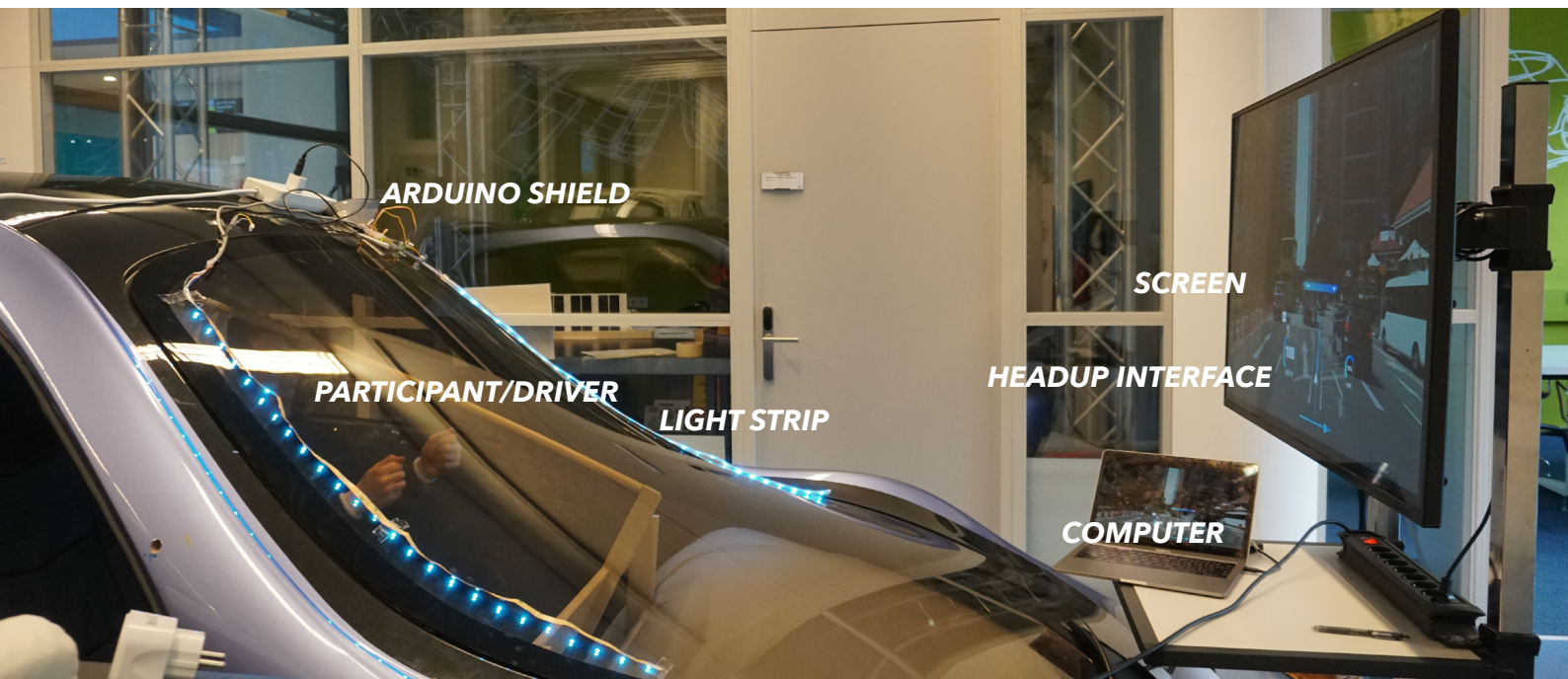
Figure 33. User test set up
