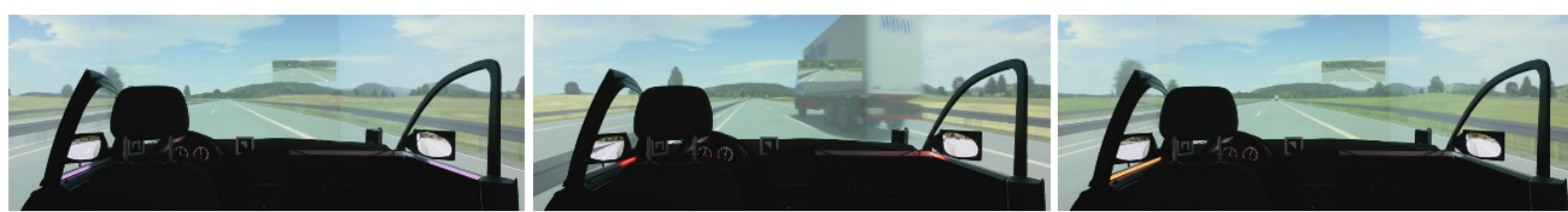
Figure 12. The implemented light pattern, embedded in out driving simulator. From left to right: accelerating, braking, changing lanes to the left. Research by Andreas etl.
