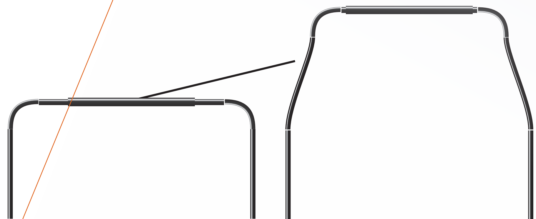
Fig.3 The two setups of the crossbar. Left the original setup. The crossbar can be moved forwards by attaching two s shaped tubes.
