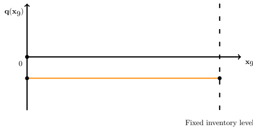
Fig. 4. Weights of the cost function are independent of the level of inventory of the retailer - formulation 1.
