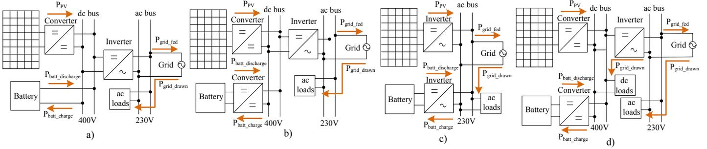
Figure 1. a) In line (1<sup>st</sup>), b) DC coupled architecture (2<sup>nd</sup>), c) AC coupled (3<sup>rd</sup>), and d) DC/AC coupled (4<sup>th</sup>)
