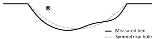
Figure 5.21: Schematic visualization of the asymmetrical features in a lateral cross section of the measured bed topography.
