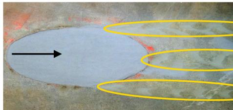
Figure 5.17: Picture from the laboratory experiment by Stenfert (2017). The sediment ridges behind the scour hole are indicated with the yellow areas.
