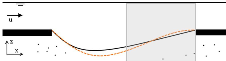
Figure 6.1: Schematization of the evolution of the bed, derived from the bed shear stress in the model results and the expected erosion near the reattachment point. The grey square indicates the area that is influenced by the bed shear stress.
