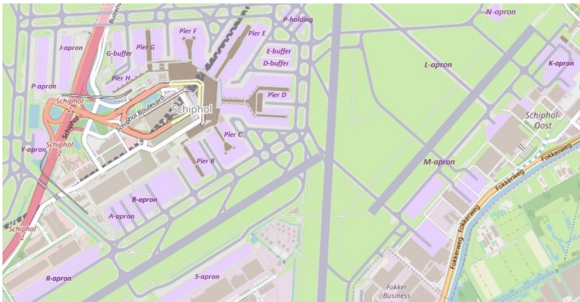
Figure 3.1: General layout of Amsterdam Airport Schiphol aprons and piers (modified from source: OpenStreetMap [49])
