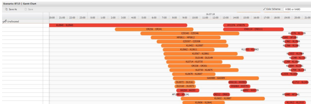
Figure 5.10: Excerpt regarding unallocated flights from allocation Gantt chart for Monday 16 July 2018, with a buffer time of 15 minutes, produced by SGA feature of BEONTRA Scenario Planning tool (WIBO flights being orange; NABO flights being red)
