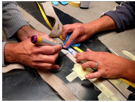
Fig. 9: Preparation of optical (glass) fibre bragg grating sensors
