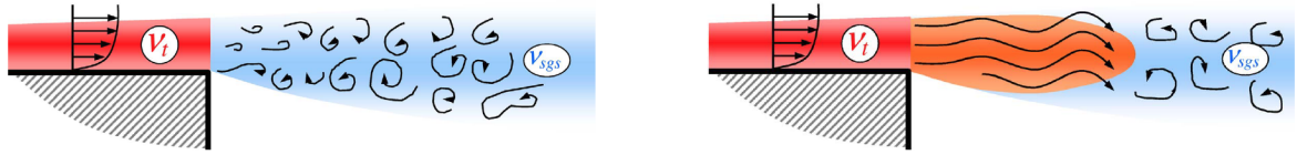
Figure 2.8: Schematic representation of the grey area problem that can be found in hybrid RANS/LES simulations. Left: ideal case. Right: real case, grey area is marked orange. By Michel et al. (2010)
