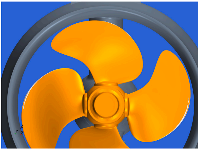
Fig. 35. Representation of the vapor volume on the blades of the second re-design, at 7 knots, with incoming flow at 15 deg angle to emulate the flow behind the ship hull.
