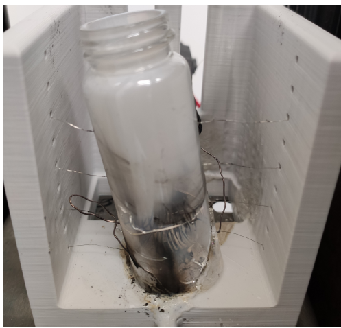
(a) Broken Jar After Injector Fire
