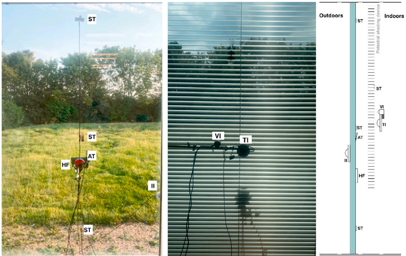
Fig. 11. Measurement setup at the facade.
