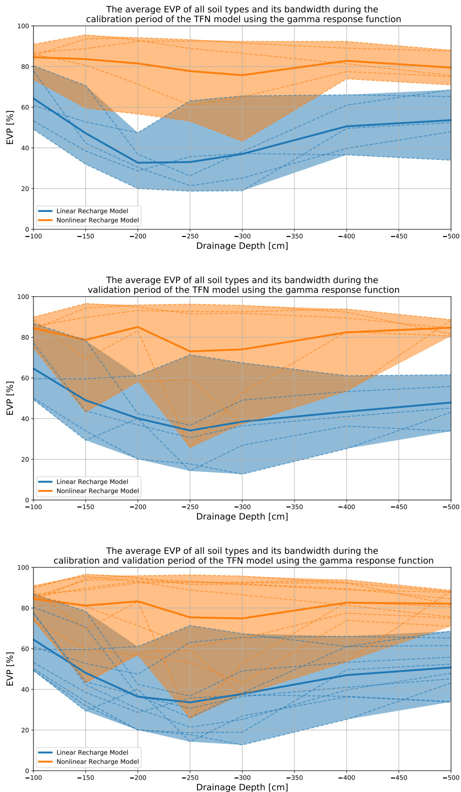
Figure B.2: The average EVP for all soil types against the drainage level for the calibration, validation period. The values for the soil types are visualised as dashed lines. The bandwidth shows the maximum and minimum EVP for any soil type for the specific recharge model. The gamma response function is used in the TFN model.
