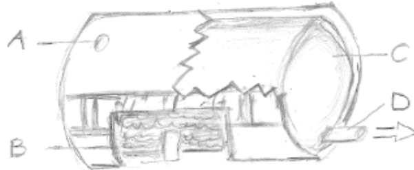
Figure 5.2: Payload Storage tank - A: Vent hole - B: Landing Gear Stowage - C: Payload Storage Tank - D: Connection Pipe to Pumping System
