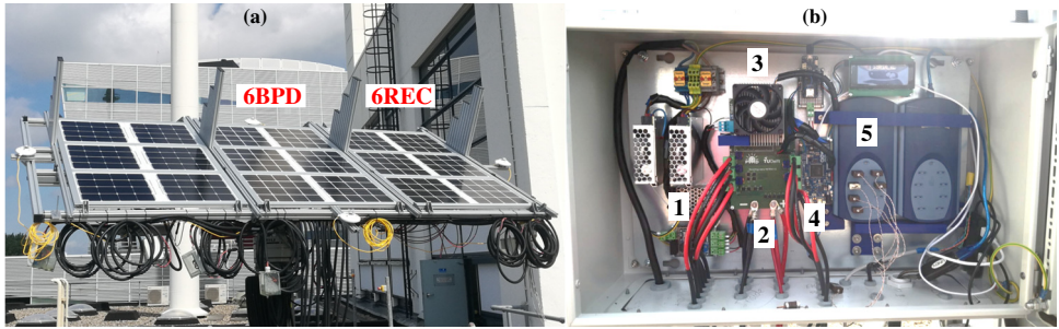
Figure 5.13: (a) Experimental setup at the PVMD monitoring station in Delft, the Netherlands. (b) Reconfiguration and sensing circuitry. (1) Power supply. (2) Switching matrix. (3) Driver circuit. (4) Microcontroller. (5) Temperature data logger.
