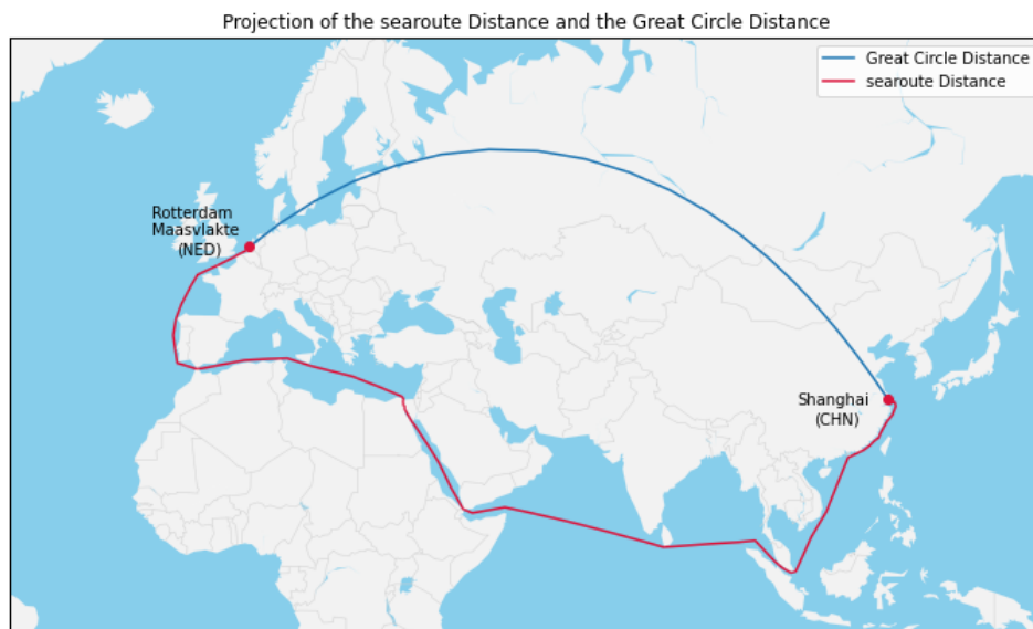
Figure 5.2: Example of the searoute distance (10580 nm) compared to the great circle distance (4834 nm) between Rotterdam Maasvlakte (NL) and Shanghai (CN)
