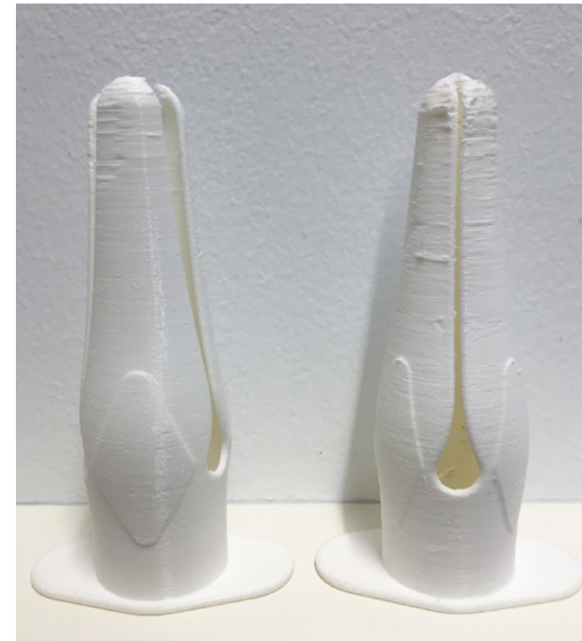
Fig. 91: TPU fails prototype with high speed
