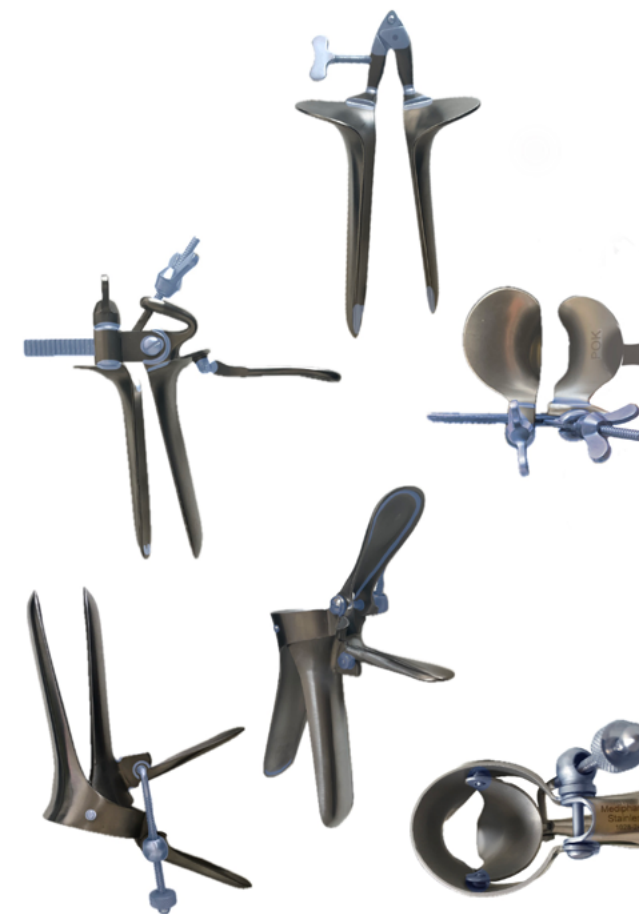
Fig. 12: Critical parts for possible trapped micro-organisms
