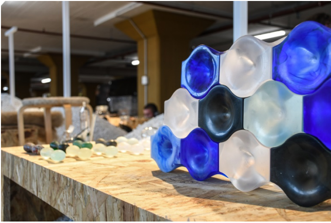
Figure 1: Prototype made by the authors of osteomorphic blocks out of recycled glass waste exhibited at the Dutch Design Week 2018.
