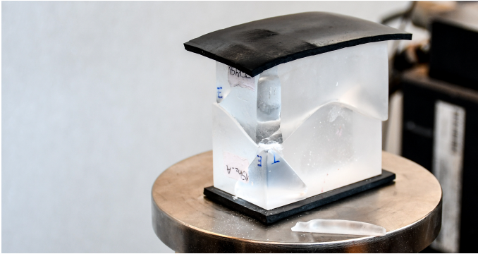
Figure 7: Failure of glass specimen without interlayer used.
