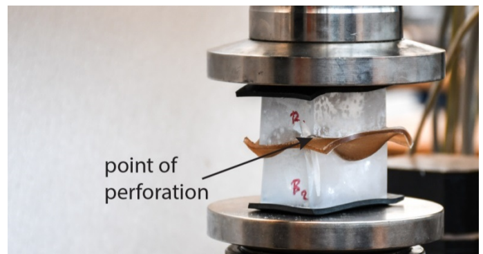
Figure 6: Typical failure at the edge of the assembly caused by the perforation/tearing of the interlayer (specimen 60A 1 )
