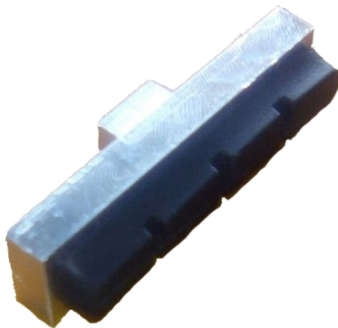
Figure 2.14: Picture of the custom pad holder with a brake pad inserted
