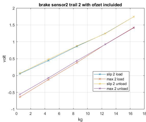
Figure F8: Plot of the voltages during loading for the first rough calibration for sensor 2 after the zero offset drift has settled. The R^2 values are: slip_{load} = 0.9981 , max_{load} = 0.9999 , slip_{unload} = 0.9976 , max_{unload} = 1.0000
