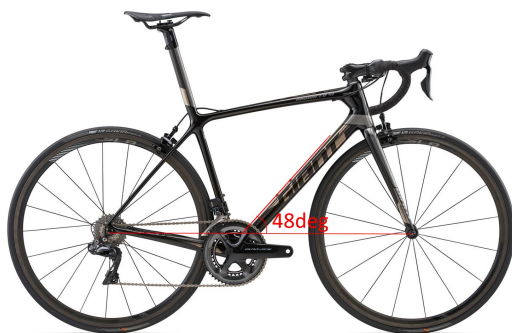
Figure K.1: Picture from the Giant website[6] with the lines used to get the down-tube angle.
