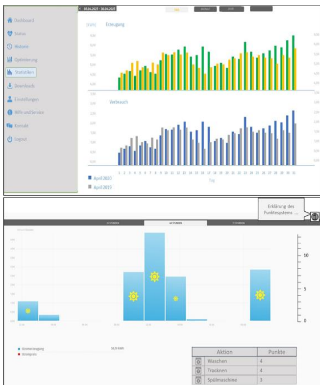
Figure 4-3: Intervention 1 for the PV- and EV-group providing simple indicators in signaling color to stimulate consumption shifts or additional consumption during PV-generation by the participants, as presented to the participants and thus, in German language, see supplementary material for further information.
