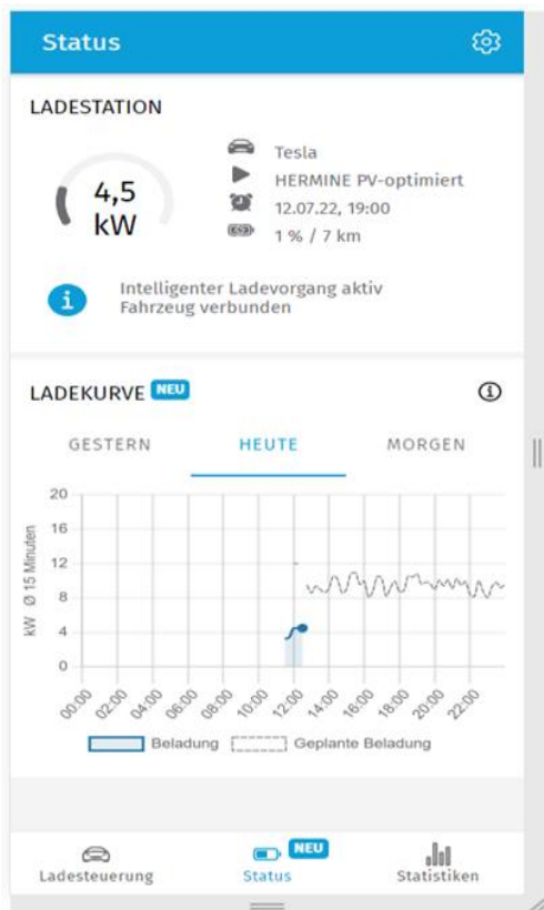
Figure Annex 10-2: Intervention 2 for the EV-group providing benchmarks of previous and current self-consumption of charging and upcoming optimized charging process
