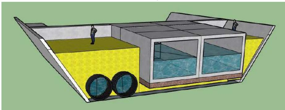
(b) 60  $m^3/s$  inlet structure at high water, beach side view
