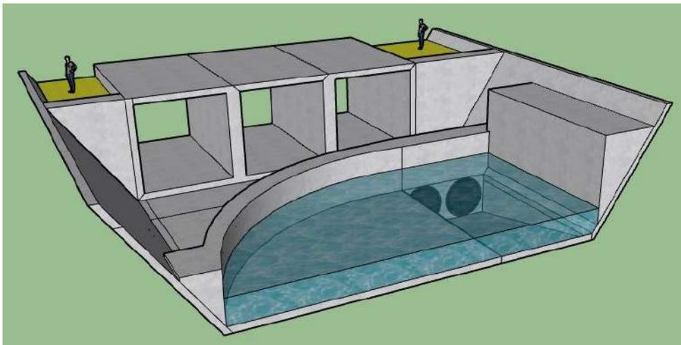
(b) River side view at culvert inlet for  $150 \text{ m}^3/\text{s}$  design capacity at low tide.
