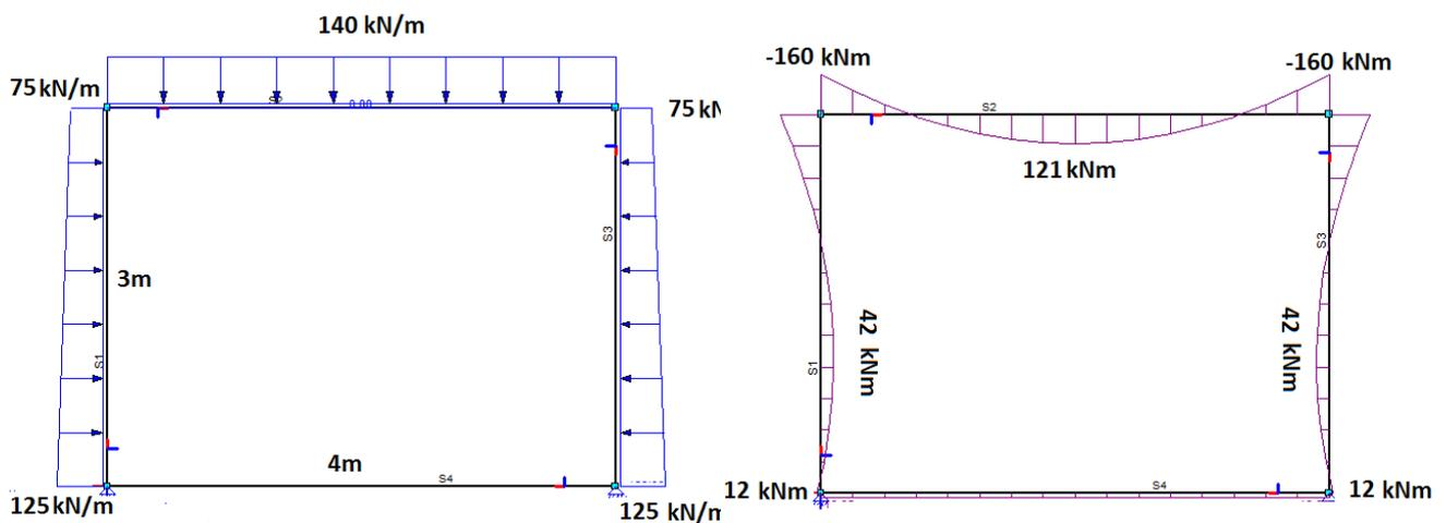
(a) Design load acting on structure for 60  $m^3/s$  design variant
