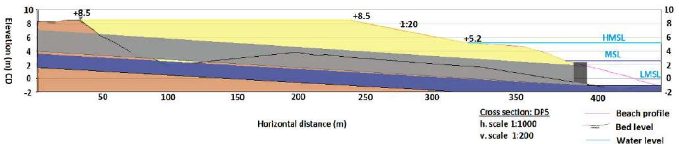
(b) Side view of position for outfall and culvert in Bella Vista beach profile.
