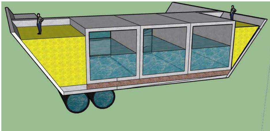
(c) Sea side view at culvert inlet for  $150 \text{ m}^3/\text{s}$  design capacity at high tide.
