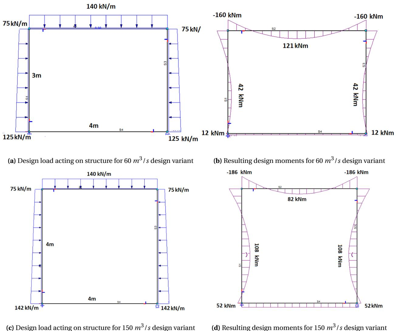
**Figure 6.64:** Forces acting on the structure for 60 and 150 m<sup>3</sup>/s design variants
