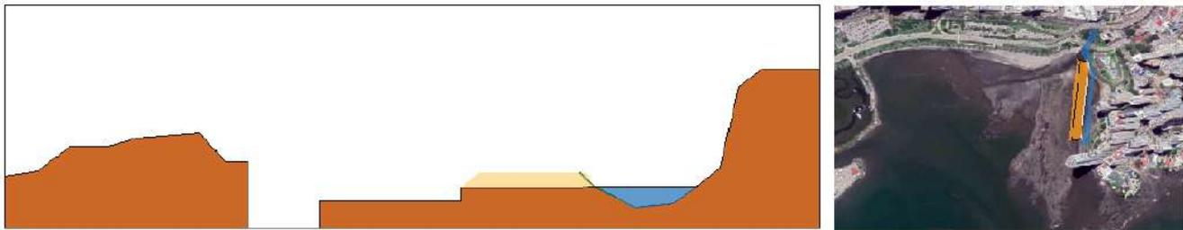
**Figure 6.50:** Phase 2: Creation of work path
