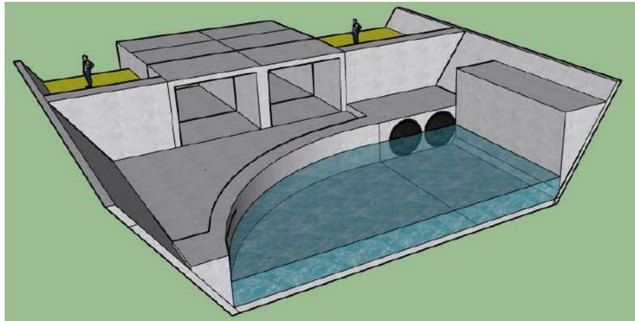
(a) River side view at culvert inlet for 60 m<sup>3</sup>/s design capacity.
