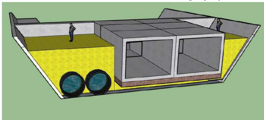
(b) Sea side view at culvert inlet for 60 m<sup>3</sup>/s design capacity
