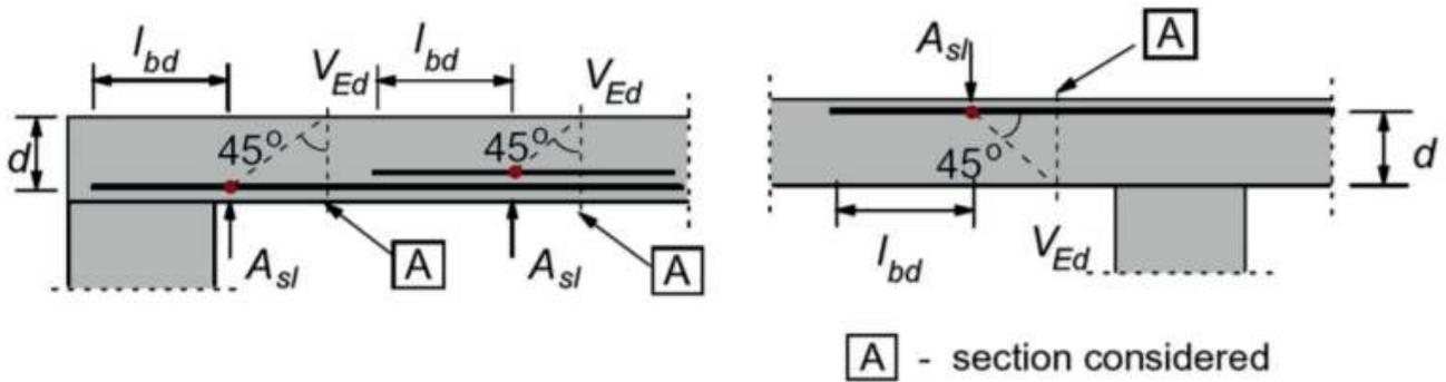
Figure 6.67: Principle of shear force without shear reinforcement(Manual Hydraulic Structures, 2019)
