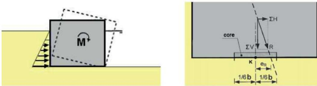
Figure 6.62: Principle of rotational stability (Manual Hydraulic Structures, 2019)
