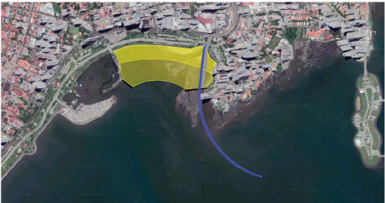
(a) Top view of the position for outfall and culvert at Bella Vista beach.
