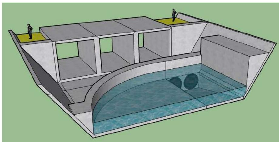
(a) River side view at culvert inlet for  $150 \text{ m}^3/\text{s}$  design capacity.
