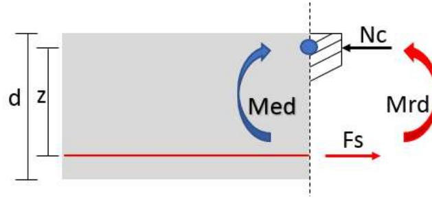
**Figure D.1:** Forces acting on cross section in the slab
