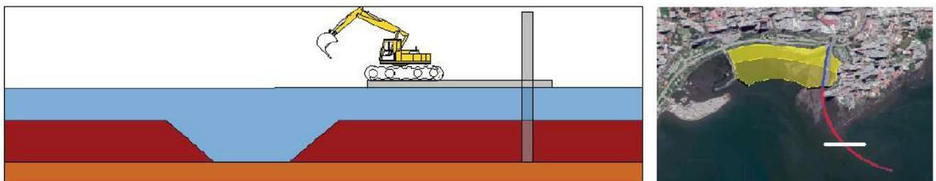
**Figure 6.56:** Phase 8: Trench dredging remaining outfall section
