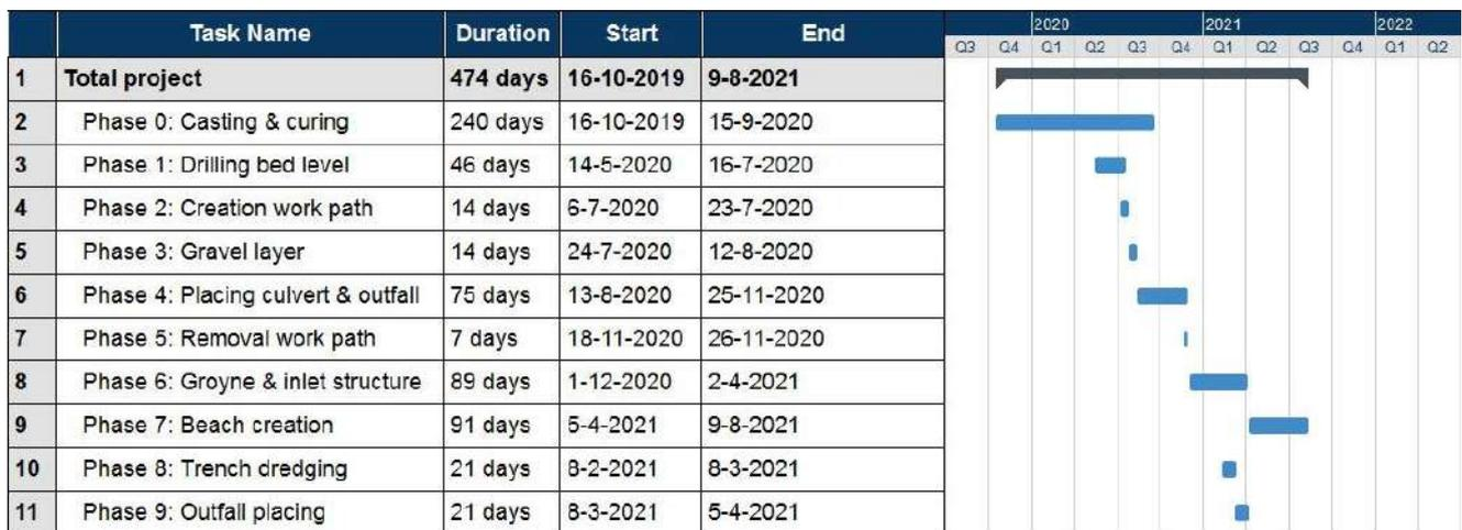
(b) Gantt chart for time planning of construction for 150 m<sup>3</sup>/s design variant (MindView)
