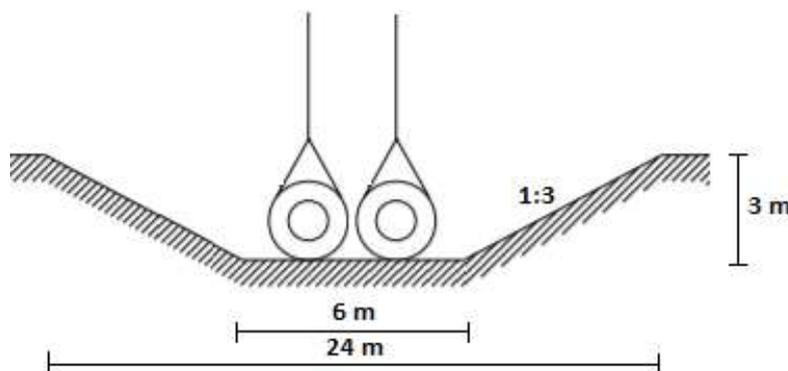
**Figure 5.41:** Cross-section of trench for the curved section of the outfall.
