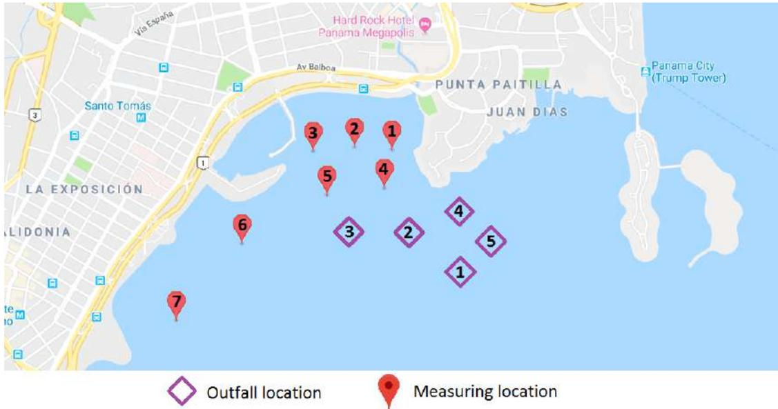
**Figure 4.33:** Visual representation of outfall locations and observation points
