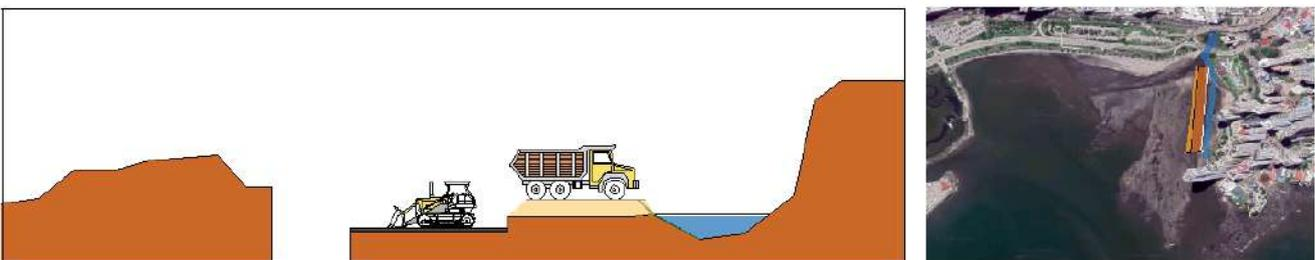
**Figure 6.51:** Phase 3: Bed leveling & placement of gravel layer
