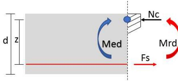
**Figure 6.65:** Forces acting on cross section in the slab
