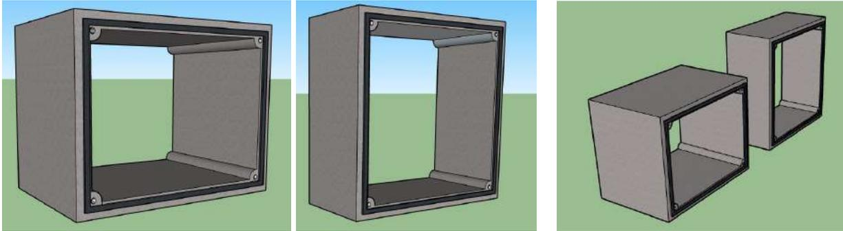
(a) Separate block section for 60  $m^3/s$  design (b) Separate block section for 150  $m^3/s$  design (c) Perspective both designs of culvert sections
