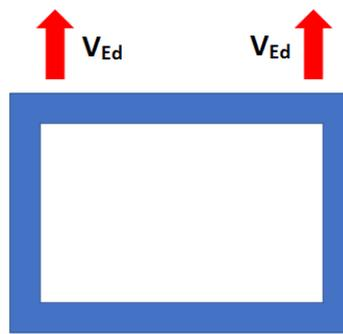
Figure D.5: Forces acting on culvert section during lifting
