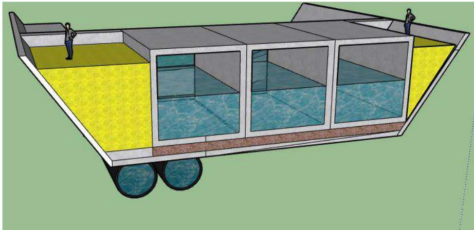
(b)  $150 \text{ m}^3/\text{s}$  inlet structure at high water, beach side view
