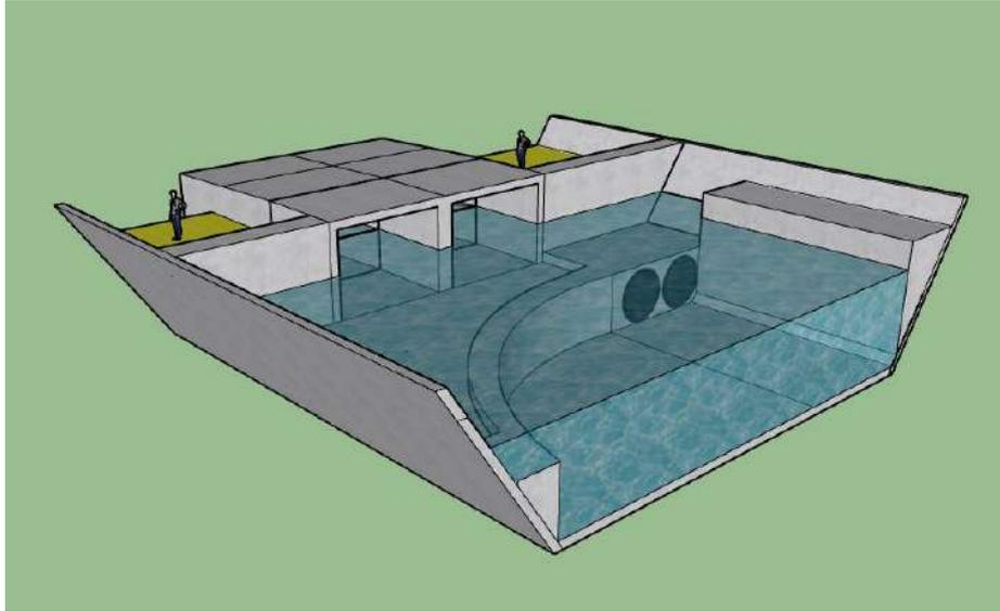
(a)  $150 \text{ m}^3/\text{s}$  inlet structure at high water, river side view
