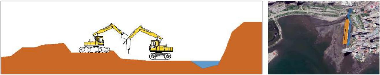
**Figure 6.49:** Phase 1: Drilling of bed level
