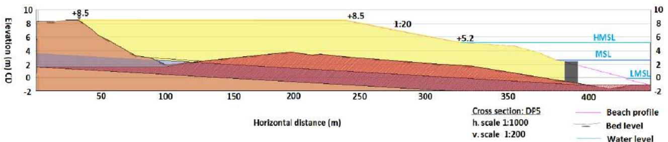
Figure 5.40: Side view for outfall, rock to be removed is indicated by the shaded red area.
