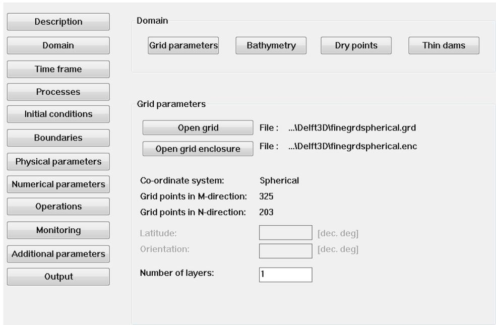
Figure C.6: Input parameters for flow model in Delft3D
