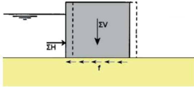
**Figure 6.60:** Principle of horizontal stability (Manual Hydraulic Structures, 2019)
