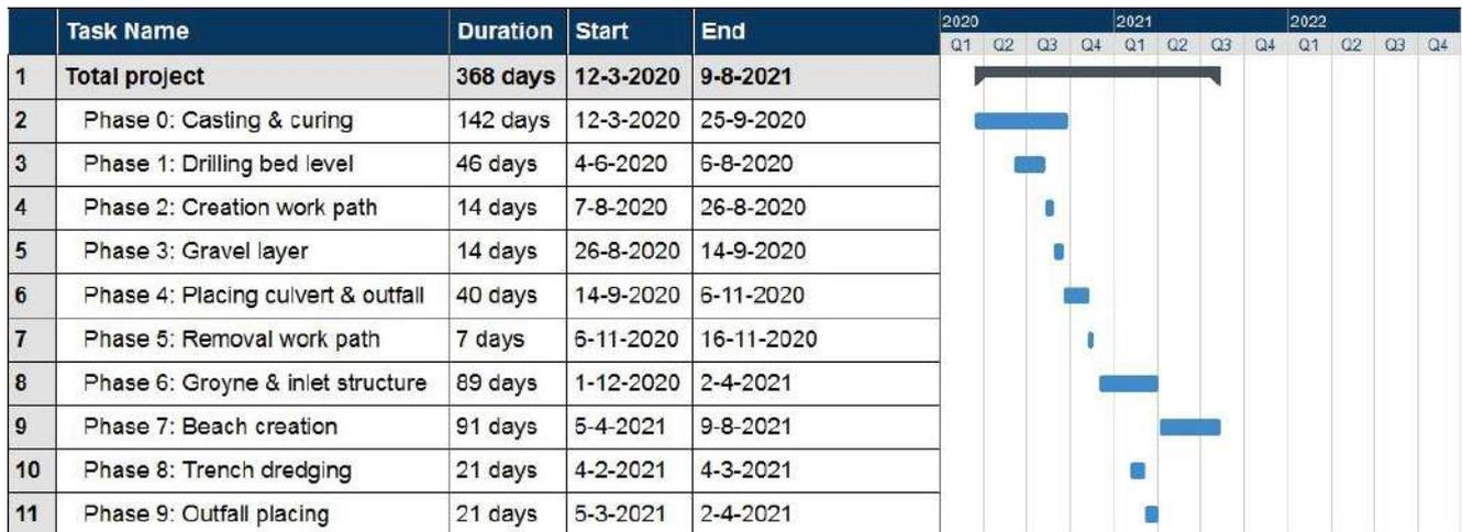
(a) Gantt chart for time planning of construction for 60 m<sup>3</sup>/s design variant
