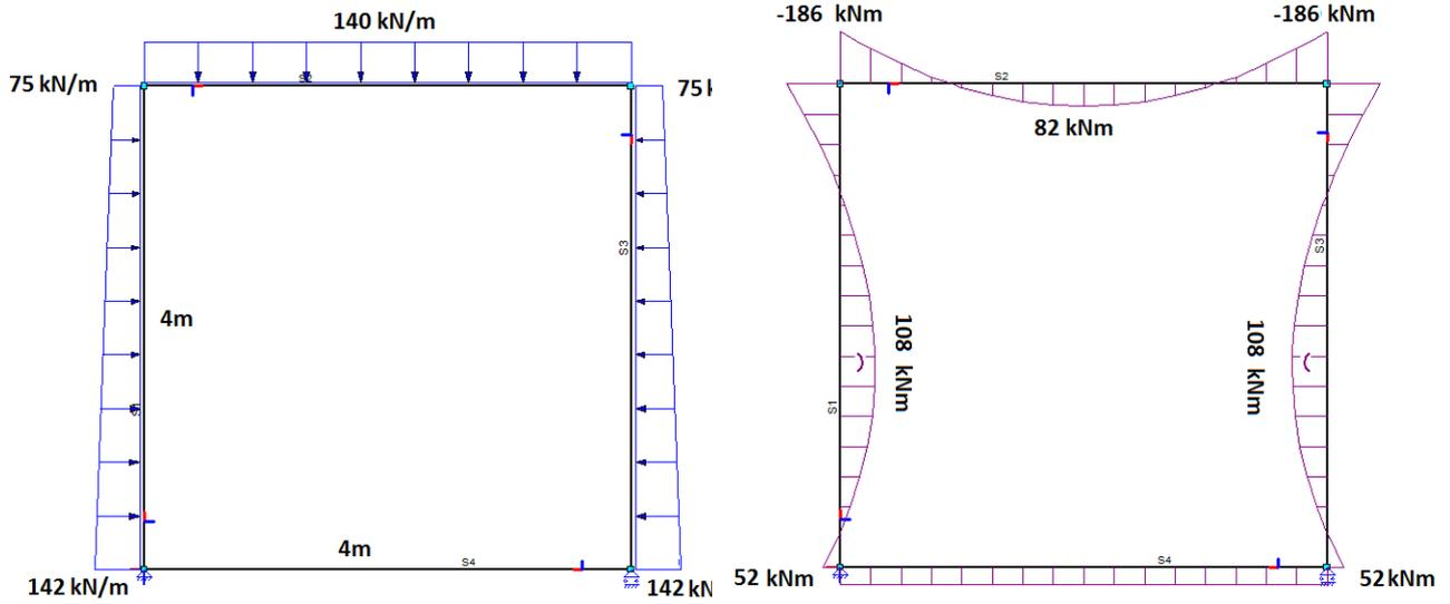
(a) Design load acting on structure for 150 m<sup>3</sup>/s design variant (b) Resulting design moments for 150 m<sup>3</sup>/s design variant
