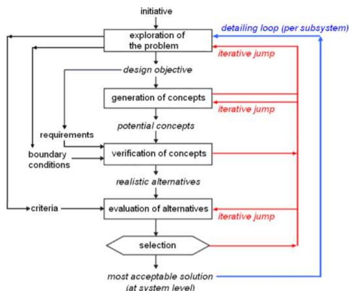
**Figure 1.8:** Engineering design cycle (Lecture notes Hydraulic structures, 2016).
