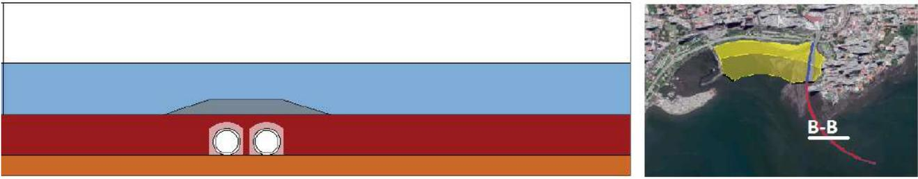
**Figure 6.58:** Phase 9: Placing remaining outfall section and backfilling
