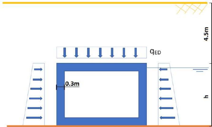
**Figure 6.63:** Forces acting on the structure
