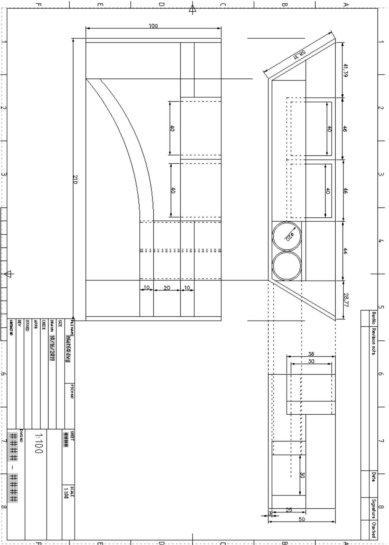
Figure E.3: Technical drawing 60 m<sup>3</sup>/s inlet structure
