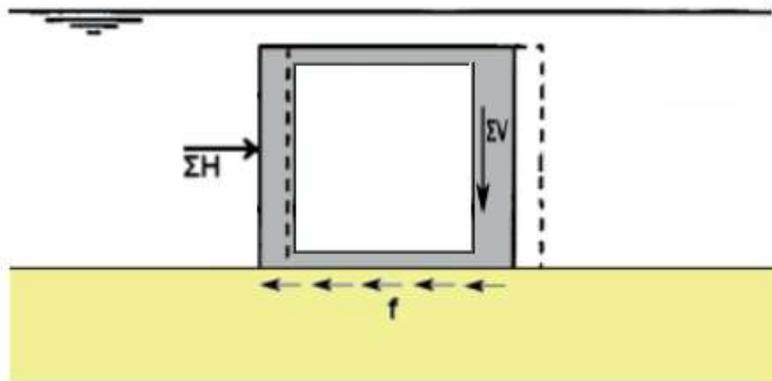
**Figure 6.61:** Principle of horizontal stability for submerged placement and tide (Manual Hydraulic Structures, 2019)
