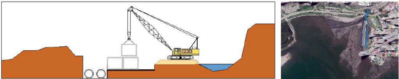
**Figure 6.52:** Phase 4: Placement of outfall & culvert sections
