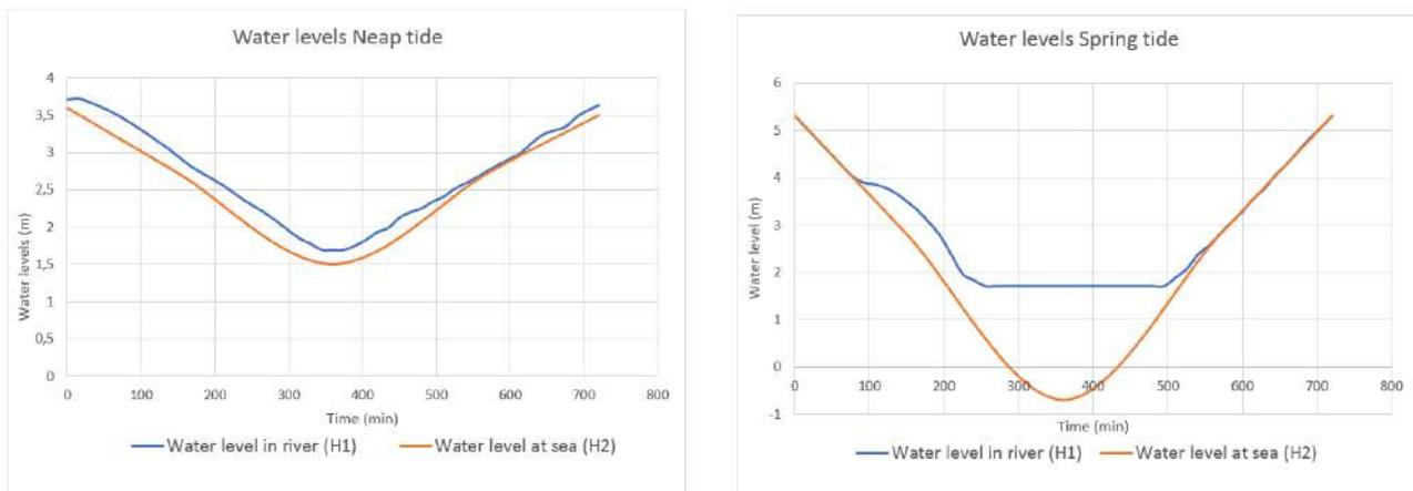
(a) Computed water levels for pipeline section of hybrid concept during neap tide (b) Computed water levels for pipeline section of hybrid concept during spring tide
