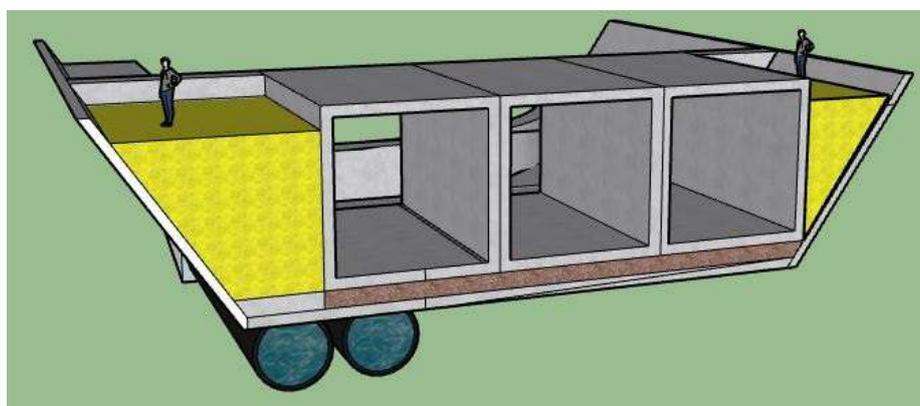
(b) Sea side view at culvert inlet for  $150 \text{ m}^3/\text{s}$  design capacity.
