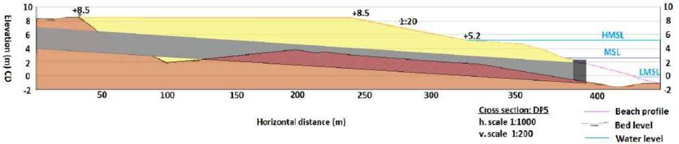
Figure 5.39: Side view for 60 m<sup>3</sup>/s culvert, rock to be removed is indicated by the shaded red area.
