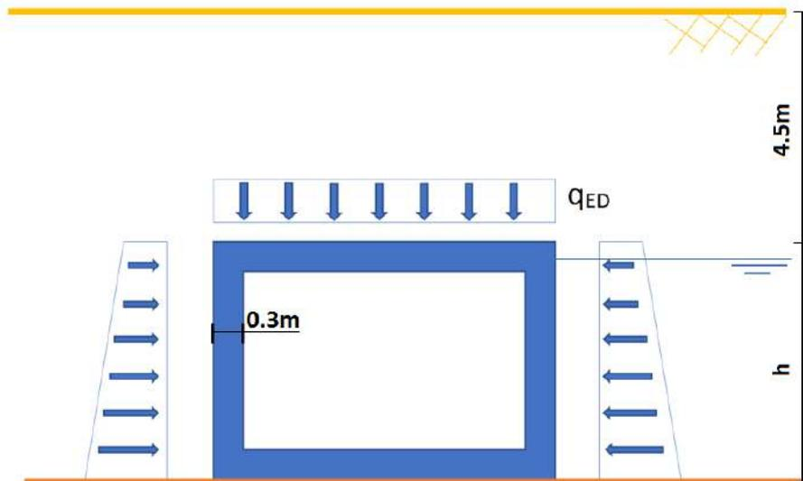
**Figure D.2:** Forces acting on the structure
