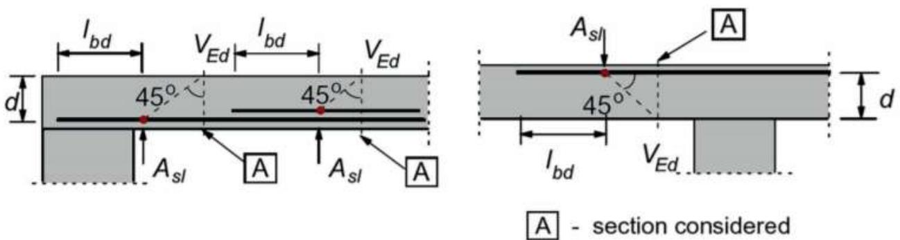
Figure D.6: Principle of shear force without shear reinforcement (Manual Hydraulic Structures, 2019)
