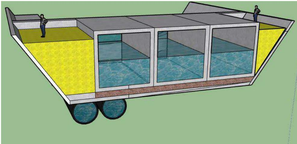
(a) Beach side cross-section of culvert inlet structure for the  $150 \text{ m}^3/\text{s}$  design capacity at a high water event.
