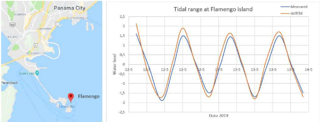
Figure 4.32: Modelled and measured tidal signal at Flamengo island
