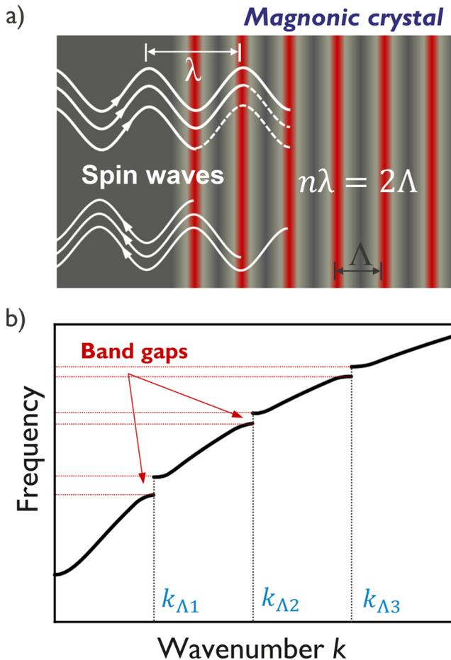
**FIG. 14.** (a) Schematic representation of Bragg reflection of spin waves (wavelength  $\lambda$ ) from a one-dimensional magnonic crystal with periodicity  $\Lambda$ . (b) Dispersion relation of a SSW mode in a magnonic crystal. The frequency bandgaps corresponding to wavenumbers  $k_{\Lambda n} = n\pi/\Lambda$  with  $n = 1, 2, 3$  are indicated.
