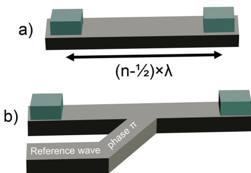
**FIG. 16.** Implementation of spin-wave inverters. (a) Phase encoding: inversion occurs by propagation along a “delay line” with a length of  $(n - \frac{1}{2}) \times \lambda$ , with  $\lambda$  being the spin-wave wavelength and  $n = 1, 2, 3, \dots$  an integer. (b) Amplitude encoding: inversion occurs by interference with a reference wave with phase  $\pi$ .
