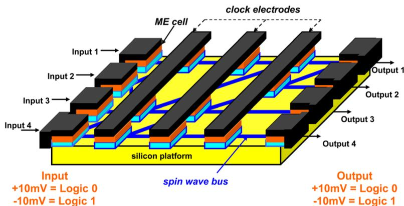
**FIG. 22.** Schematic view of a spin-wave circuit with nanomagnet-based cascading. Spin waves propagating between nodes of the circuit switch the magnetization of bistable nanomagnets. Clock electrodes then provide trigger signals to launch spin waves from one node to the next in the following clock cycle. Reproduced with permission from A. Khitun and K. L. Wang, *J. Appl. Phys.* **110**, 034306 (2011). Copyright 2011 AIP Publishing LLC.
