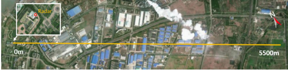
FIGURE 12 Experiment scene: The radar is set on the top of the building and the small drone flies along the radial direction of the radar within 0–5500 m
