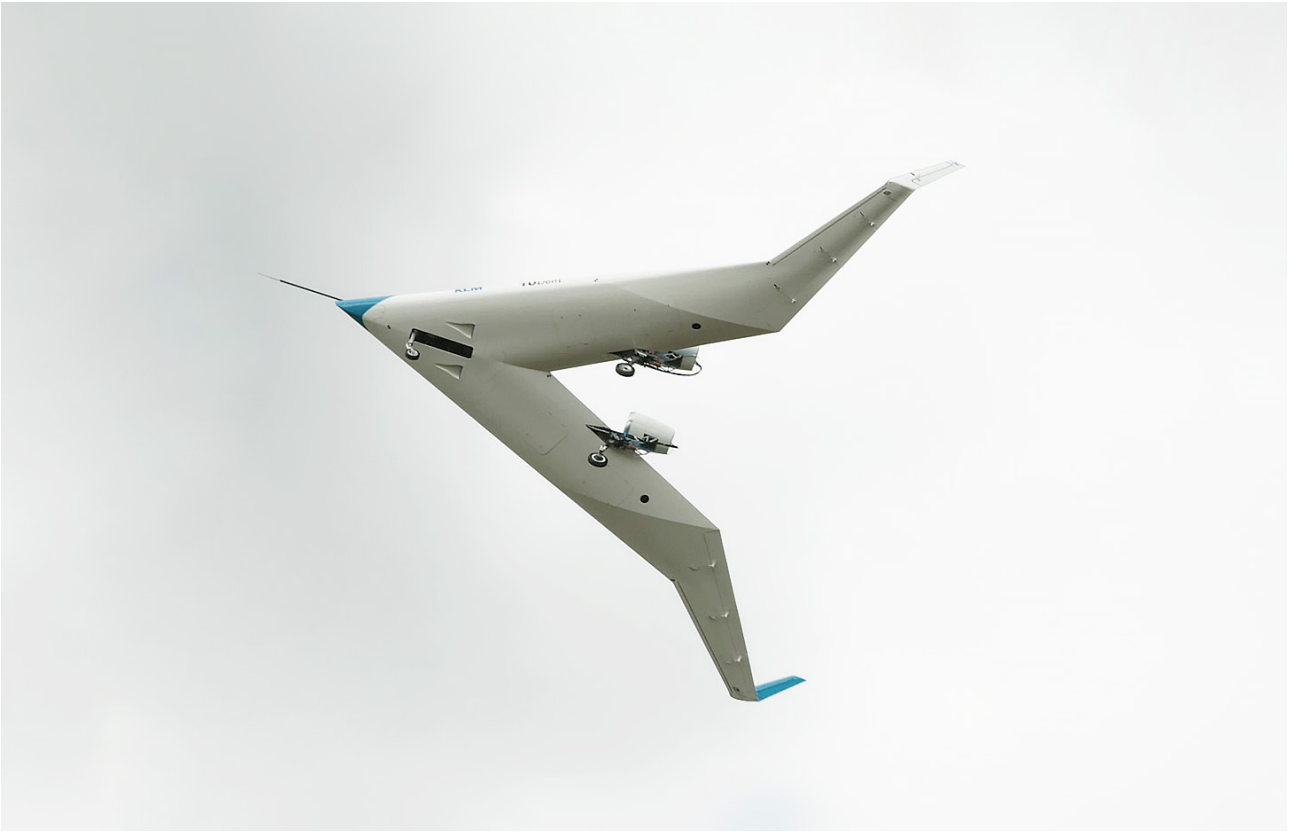
Figure 10: First flight of the 4.6% Flying V sub-scale flight testing model, Fassberg Air Base, July 14, 2020.
