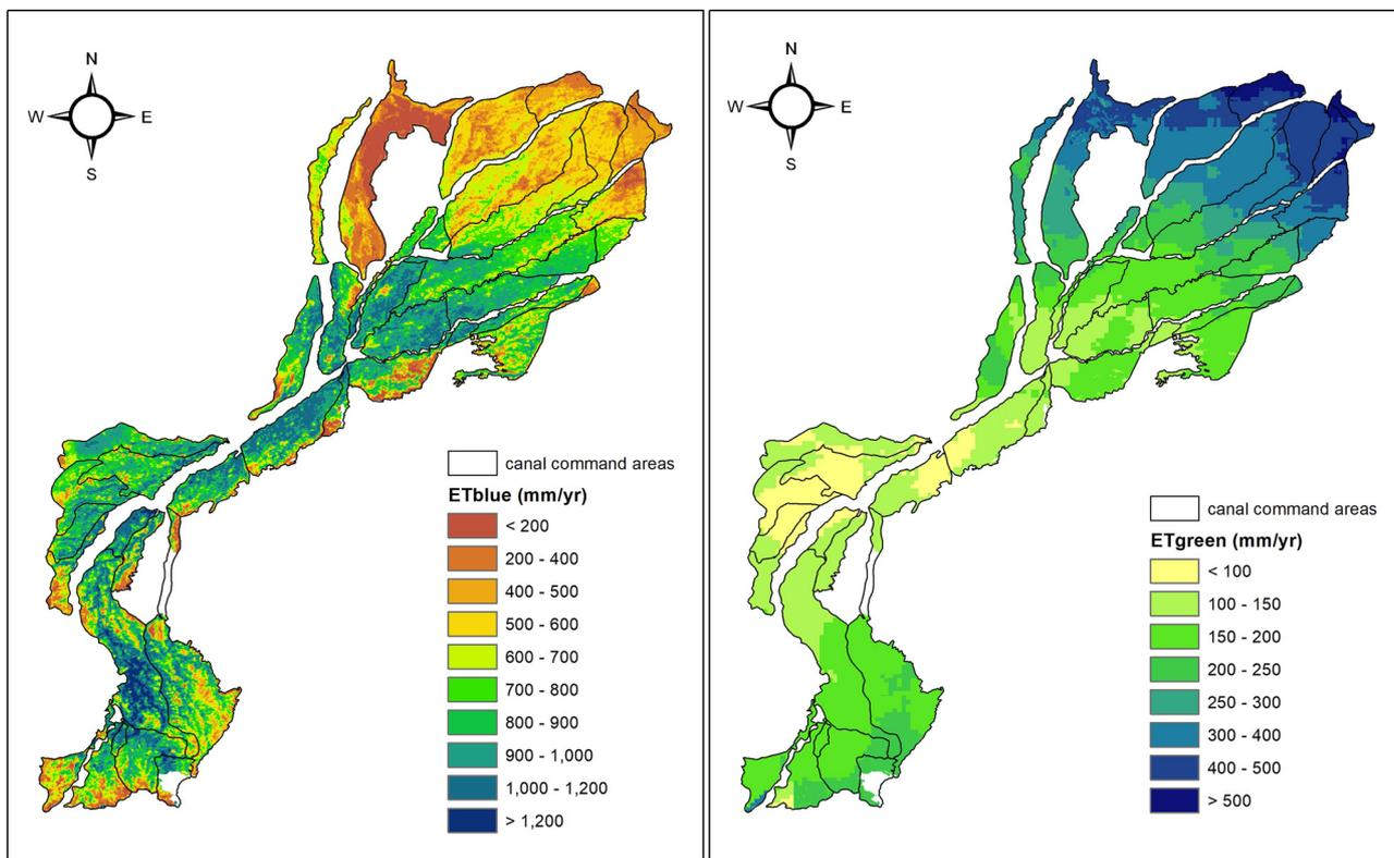
Fig. 5. Annual blue water evapotranspiration ( $ET_{blue}$ , left) and green water evapotranspiration ( $ET_{green}$ , right) across the Indus Basin Irrigation System, averaged for 2004 – 2012. (For interpretation of the references to colour in the Figure, the reader is referred to the web version of this article).
