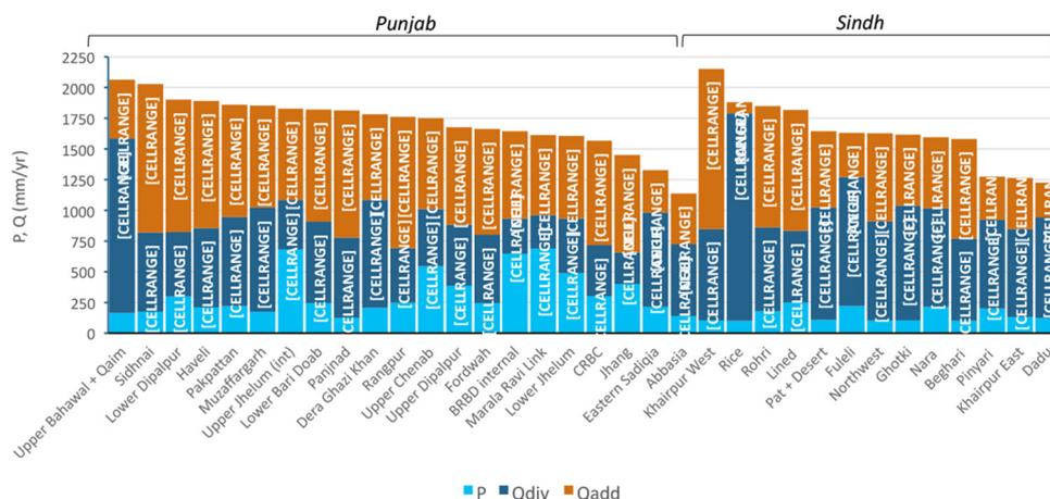
**Fig. 8.** Different sources of water for each canal command area: precipitation (P), canal water ( $Q_{div}$ ), and additional supply ( $Q_{add}$ ). Percentages indicate the extent to which water use in each command area depends on sources other than rainfall or water diverted to the main canal.
