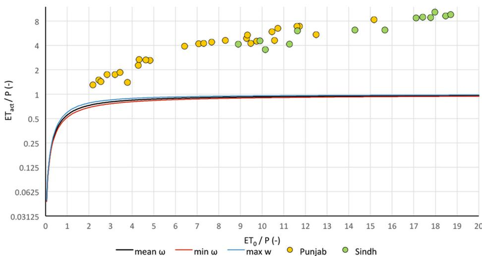
**Fig. 4.** Ratios between actual evapotranspiration ( $ET_{act}$ ) and precipitation ( $P$ ), and between reference evapotranspiration ( $ET_0$ ) and  $P$ , of canal command areas in the Indus Basin Irrigation System for the 2004 – 2012 period. The presented Budyko curves are calculated with  $\omega$  values of 1.88, 1.76, and 2.05, corresponding with command area-level mean, minimum, and maximum values, respectively.
