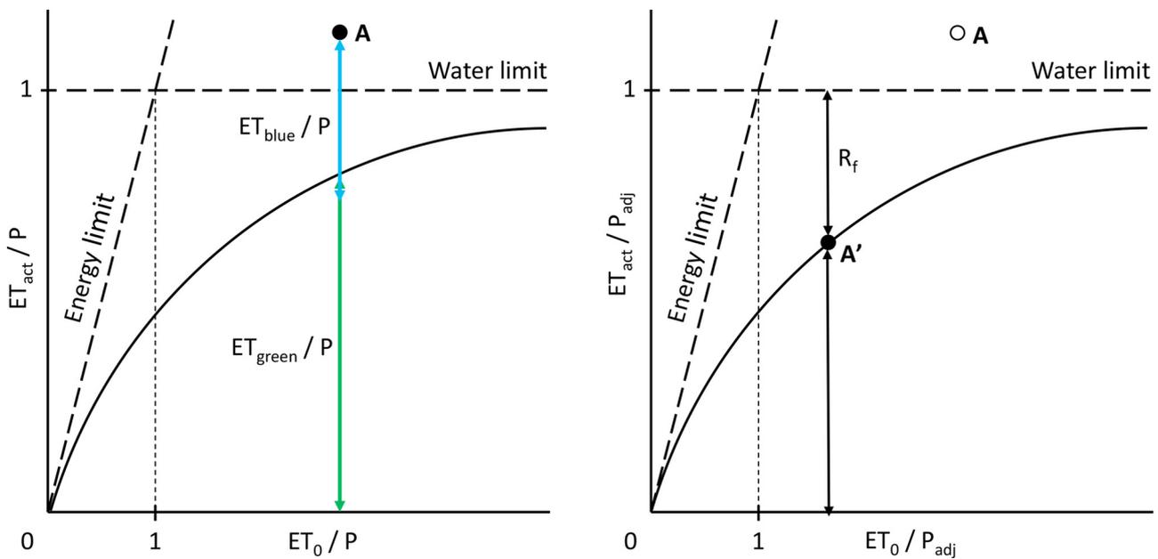
Fig. 2. Location of an irrigated basin (A) in the Budyko framework when considering rainfall (P) as the sole term on the supply side (left) and its new location A' on the Budyko curve when considering all sources of water (P<sub>adj</sub>, right). ET<sub>act</sub> and ET<sub>0</sub> refer to actual and reference evapotranspiration, respectively.
