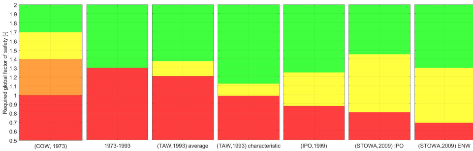
Figure 1.1: Overview of the required global factors of stability for regional dykes (1973 to the present day). In red (lowest), stability factor not acceptable; in orange, more detailed research is required; in yellow, acceptable depending on the material and economic value of the polder; and in green (highest), acceptable.
