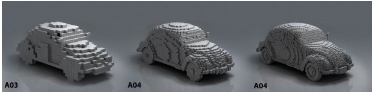
Figure 3.3: Representation of voxelization, from left to right large voxels to small voxels (Venuti, 2103)
