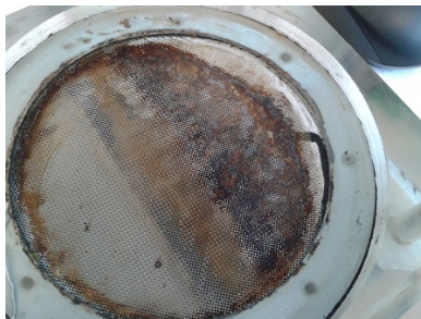
Figure 3.6: Corroded anode of a cell that contained a LiNO 3 solution.
