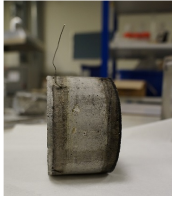
Figure 3.24: Specimen with embedded titanium mesh. The wire coming out of the specimen on the left is from the embedded mesh.
