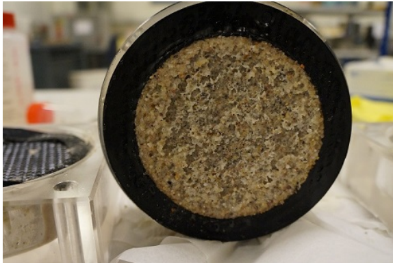
Figure 3.17: The anolyte surface of the specimen \text{LiNO}_3 7.8 M 4w.(I). The surface was deteriorated by the acidic anolyte solution.
