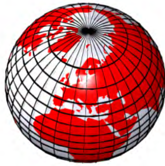
Figure 2.5: Traditional DGGS - The surface of the Earth is divided by meridians and parallels.
