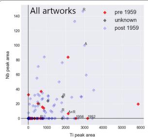
**Fig. 7** Scatter plots of niobium K vs titanium K peak areas of all artworks (average value of the spectra taken from white areas) colored by date, related to the date of introduction of the chloride process (1959) and labelled for unexpected dates or, if known, the pigment crystal structure
