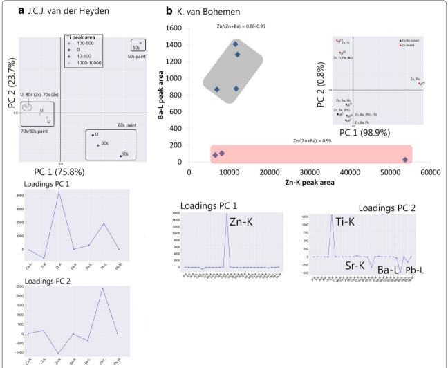
**Fig. 6** a PCA scoreplot and loadingplots (PC1 and PC2) of 11 paintings by J.C.J. van der Heyden, averaged over the spectra of the white areas. PCA was done taking only the white elements (Ca, Ti, Ba, Zn, Pb) into account. **b** Bivariate Ba-L vs Zn-K analysis and PCA scoreplot of 7 paintings by van K. van Bohemen, averaged over the spectra of white areas
