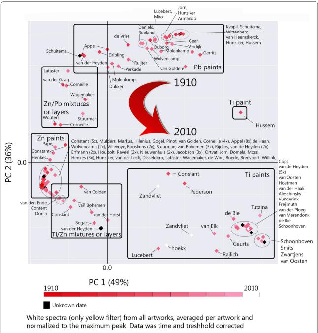
**Fig. 4** PCA scoreplot of all artwork averaged for spectra taken from white areas and normalized to maximum. The scores in the plot are boxed by type of paint, colored using a red gradient by decade and labeled by artist. The origin lines are indicated in black. This figure can be interpreted as a reference roadmap of how different white pigments have been used throughout the 20th century. The time arrow represents the identified trend, despite several exceptions in the lead cluster
