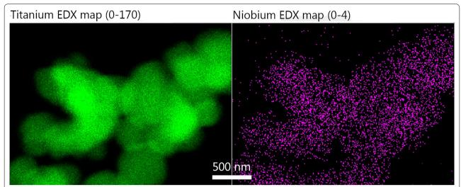
Fig. 8 STEM-EDX map of Titanium dioxide pigment containing niobium impurity (powder: RCE9649 from RCE reference collection). The intensity range of EDX detection for Ti and Nb respectively are provided between brackets in the figure header
