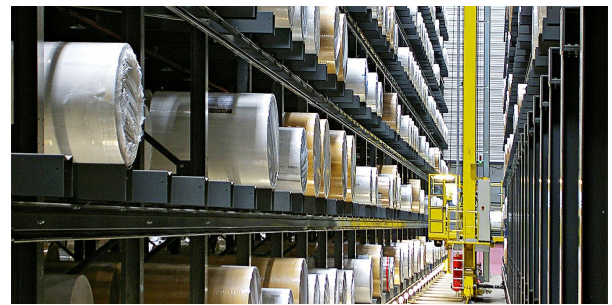
(b) Aisle captive stacker crane (chain 2021)
