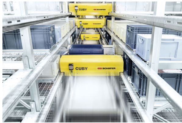
Figure 4.3: Example of an aisle-based shuttle ASRS (SSI Schäfer 2021)
