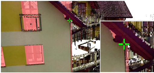
Figure 6: Shape-assisted point picking performed on a shape cluster representing the foreground wall. Note that the cross hair does not jump to a point in the background even if it is closer to the cursor in screen space.
