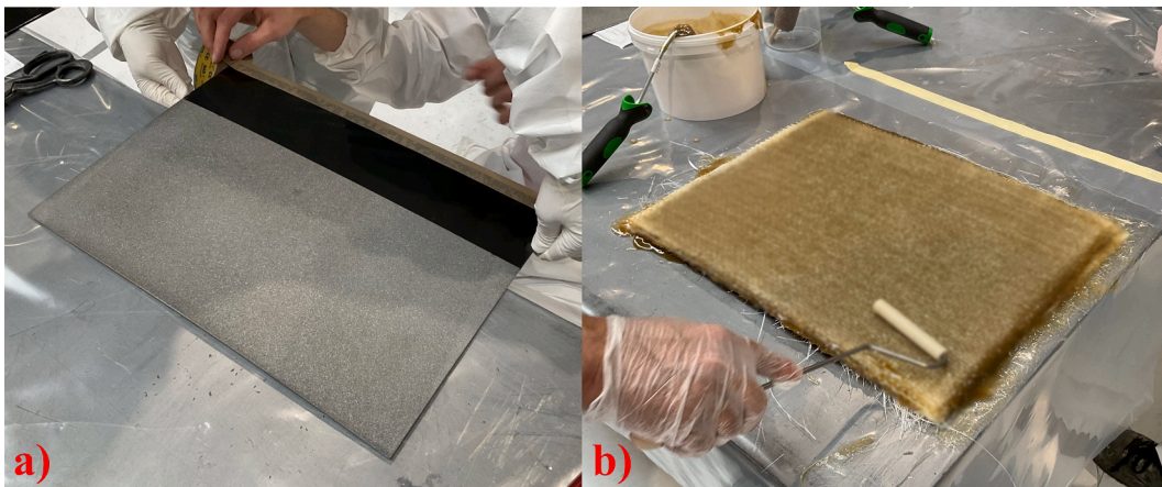
Fig. 4. Manufacturing of the composite-steel bonded plate: a) the steel plate with a pre-insert; b) the hand lay-up lamination process.
