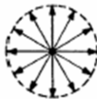
Figure 2.8: Directivity pattern of a monopole source
