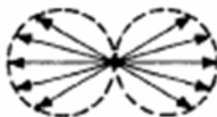
Figure 2.9: Directivity pattern of a dipole source
