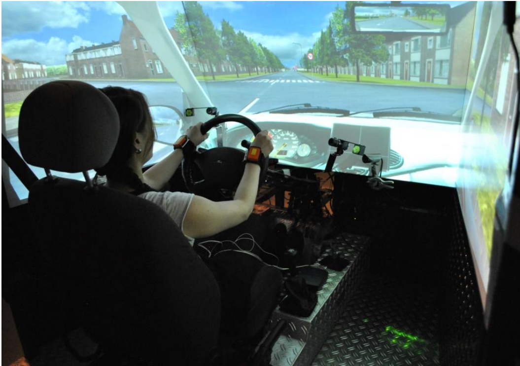
Fig. 1. One of the experimenters in the driving simulator, with inertial sensors and eye tracker.
