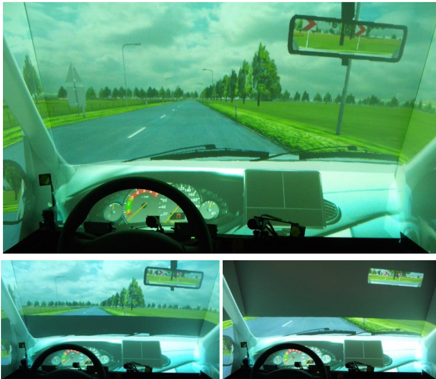
Fig. 1. Photos of the driving simulator; Top = control condition (C); Bottom left = near view (NV), all sight above 5 degrees below the horizon was blanked; Bottom right = far view (FV), all sight under 4 degrees below the horizon was blanked.
