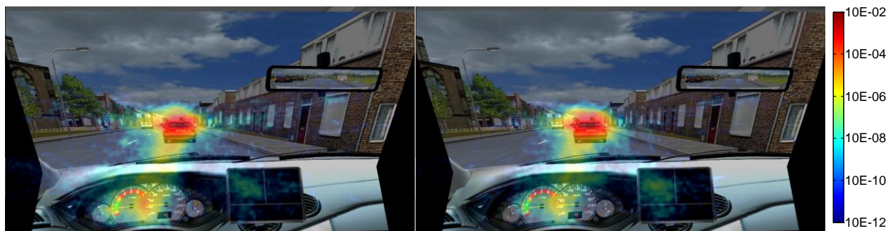
Fig. 9. Heat map of gaze probability density during car following in the No time pressure (NTP; left) and Time pressure (TP; right) sessions, overlaid on a screenshot of the simulator display. Gaze distributions were determined by aggregating gaze data from car following sections of all participants in one-by-one degree bins and are shown on a logarithmic scale.
