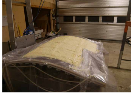
FIGURE 6.11 Curing of the HDPU foam on the flexible table
