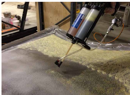
FIGURE 6.16 Applying the HDPU
