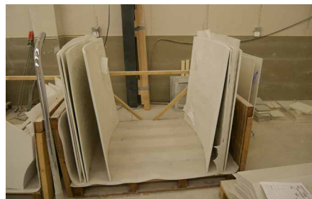
FIGURE 6.31 Finished cast panels for ring 1 and ring 2.
