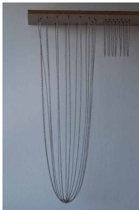
FIGURE 6.27 Catenary model of the initial design.
