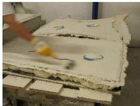
FIGURE 6.18 The finished sprayed GFRC being compressed with rollers to mitigate voids and air-bubbled in the GFRC.
