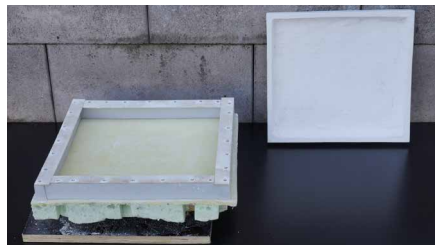
FIGURE 6.25 Intermediate mould with high edge-return
