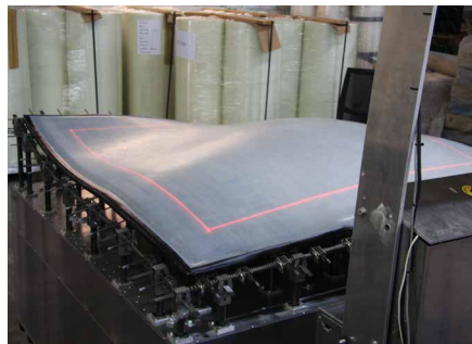
FIGURE 4.9 Digital flexible table with actuators and membrane positioned to give a free-form surface
