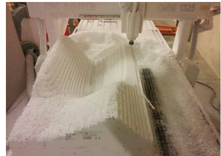
FIGURE 4.8 Concrete mould milled by a CNC machine
