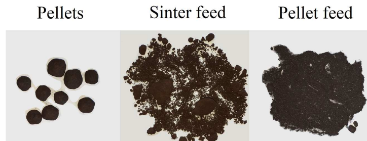
Figure 3-3. Various size range in iron ore products; pellets, sinter feed and pellet feed [21]
