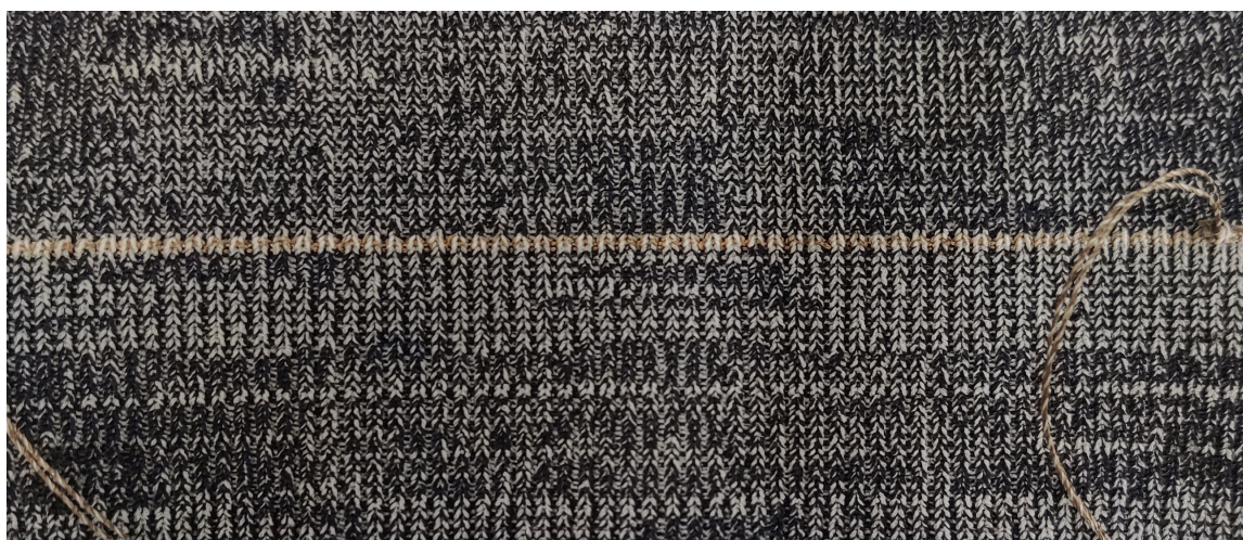
figure 1.1.1 weft knitted sensor by the TU Delft
