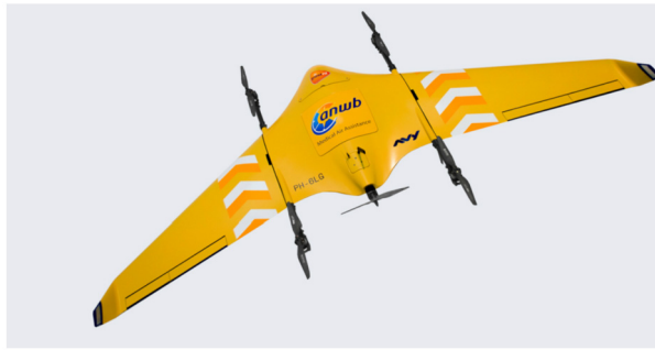
Fig. 1. A quad-plane example: Avy for medical delivery [1].
