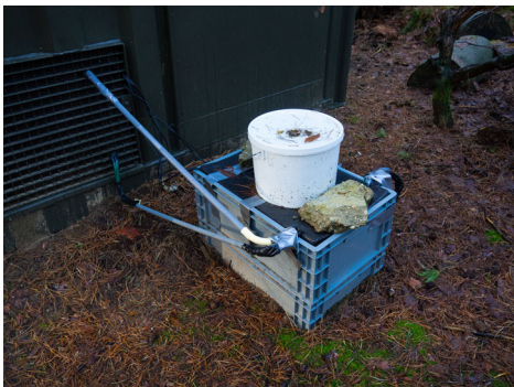
(e) The two calibration baths are stacked upon each other, the upper heated with a motor and the lower kept relatively cool at ground temperature.
