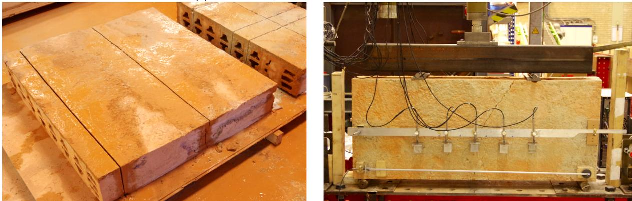
Figure II.1 (3.1&3.3). In-plane bending samples cut from NeHoBo panel (left) and four-point bending test set-up for in-plane bending of NeHoBo floor sample (right).
