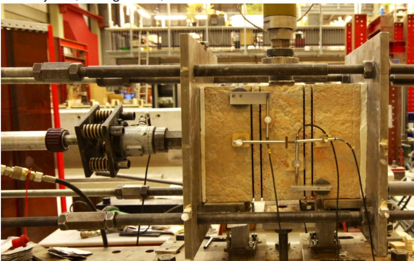
Figure II.3 (3.15) Shear test set-up with NeHoBo shear sample of which the concrete is cut at the location of the mortar joints to eliminate the contribution of the concrete layer.
