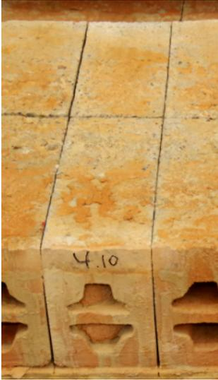
Figure 3.20. Single brick cut from NeHoBo floor panel.
