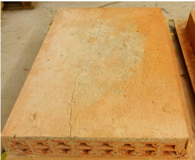
Figure 3.4. NeHoBo floor panel number 2 showing a severe crack in the top concrete layer.
