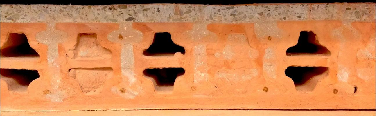
Figure 1.2. Section of NeHoBo floor sample.
