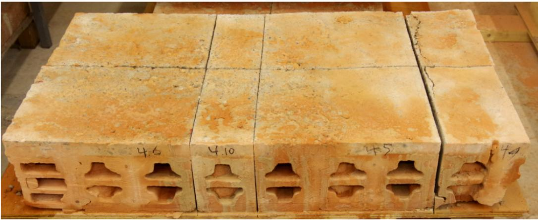
Figure 3.14. Shear samples cut from NeHoBo floor panel.
