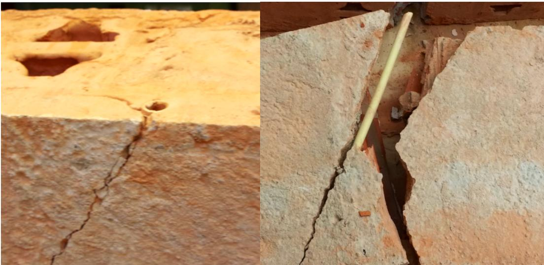
Figure 3.5. Sample TUD\_NEH-2-2 (left): crack in concrete layer at location of tube for electrical wiring in the top concrete layer. (right): Cracking of the concrete layer along the initial crack in the concrete layer.
